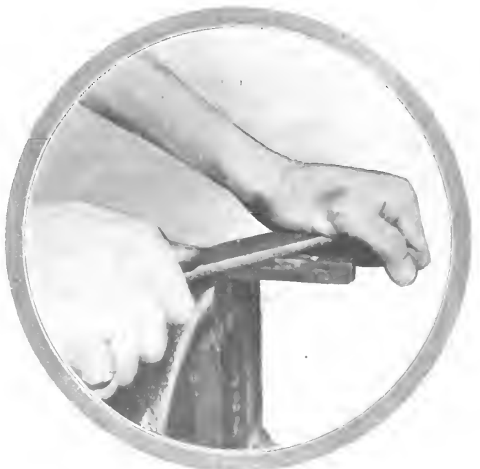
Fig. 2—Illustrating the method of filing the burr from clutch key
